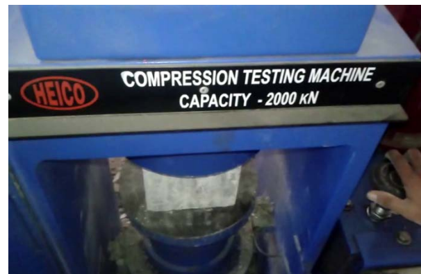
Fig. 2: Testing of cube
